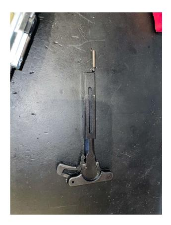
Lift up the rear of the charging handle and remove, complete with the return spring
