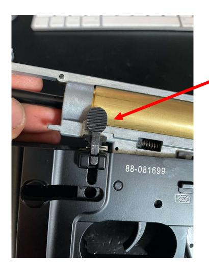
Note. Selector plate may detach if previously fitted with an ETU. If using the original trigger switch, then it will stay in place until removed.
