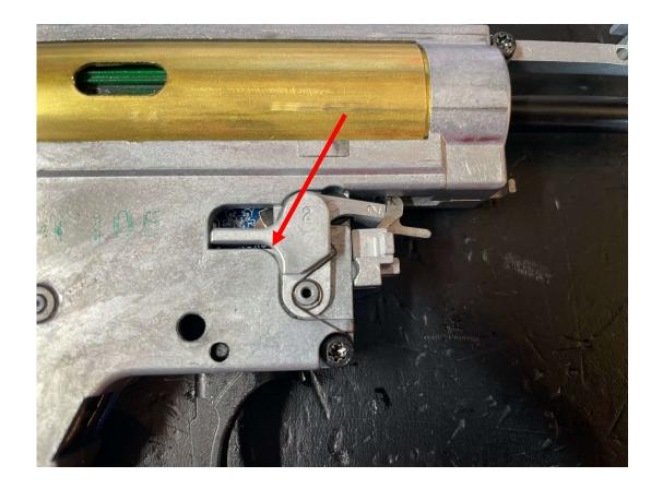
Reassemble the gearbox and bolt catch mechanism. You can see how it operates the bolt stop microswitch arrowed. Easiest way to refit this mechanism is to lay the spring in place and then gently insert the retention screw part way before hooking it it to position. Then tighten the screw down.
