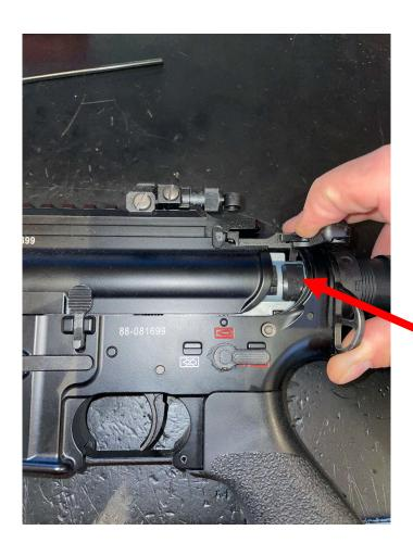
Note: there is a plastic spacer either side of the gearbox assembly that should be removed now to avoid losing them. These spacers are labelled L and R and fit on the rear tabs on the upper
