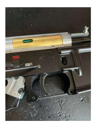
Push through the trigger pin and remove.
