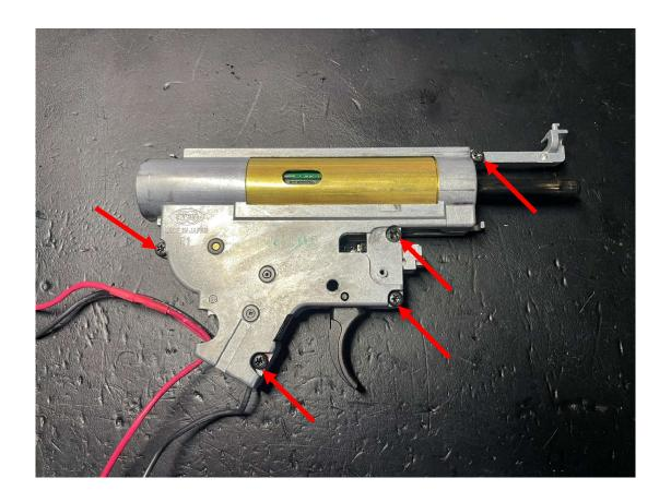
Remove arrowed screws and separate gearbox halves carefully. This rifle was fitted with an ETU that had failed totally.
