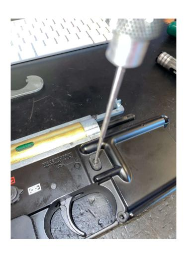
Unscrew and remove the magazine release catch and spring using a 1.5mm Allen key
