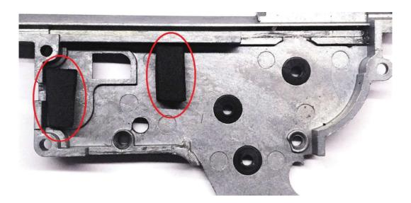
There are 2 foam pads to fit in the other half of the gearbox to keep pressure on the unit when box is closed. Use some IPA to clean the box before sticking these in place.
