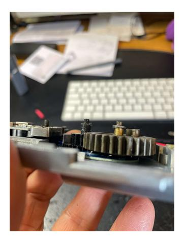
Taking the sector gear and retained shims. Ensure there is clearance between it and the unit sensors.
