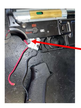
The motor can now be disconnected and removed. Note: pay attention to the wire orientation and routing within the grip. The wiring shown is reversed from standard due to the fitted ETU.
