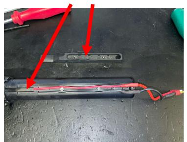
Push slightly forward and lift the rear of the assembly. The long spring is held in place by a small tabbed washer which can be easily lost so watch this as you lift the assembly out.
