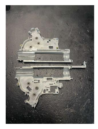
Remove the gearbox components. If re using the gears, then ensure you keep them on the correct gears to save a job later. Make sure none are stuck to the bushings! This gearbox has steel bushing although TM standard ones are plastic.
