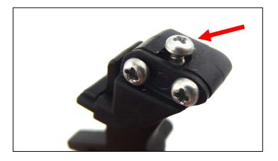
Make sure adapter will not hit sector gear teeth, otherwise grind the adapter to fit better on the trigger
