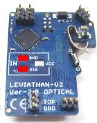
**WARNING:** Installation requires advanced soldering skills! Wires can't touch other pads and components on the board. Damage to the Leviathan will void the warranty!
