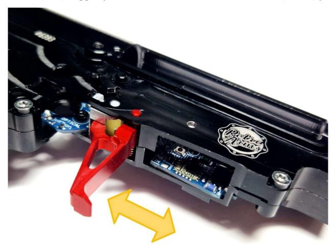
Insert adjustable trigger into the gearbox - upper part first. Then push the bottom part into the gearbox too.
