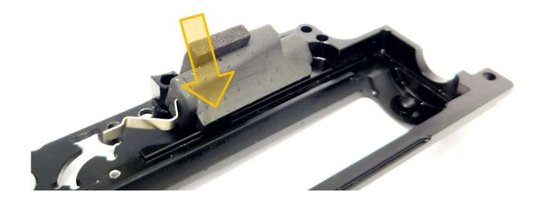
Lube the bottom part of the spring and trigger end with a small amount of grease. It will make a smooth trigger pull.
