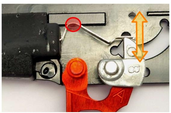
When you find the right place for the adjustable trigger, clean the gearbox shell in this area from any dirt or oil. Remove cover from this sticker and place an adjustable trigger into the gearbox.
