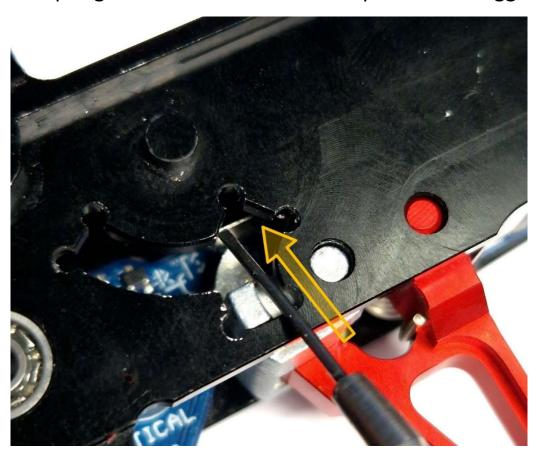
It is normal the spring is about half way on the trigger. It is for reducing the drag when the trigger returns to the default state.
